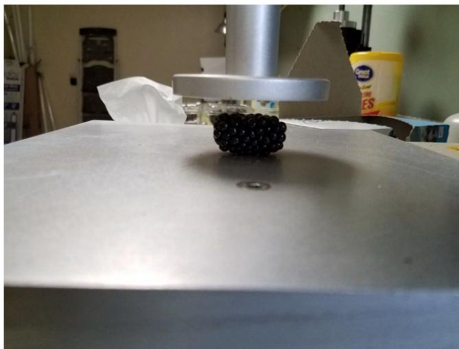
Fig. 2. Firmness (N) was measured by compression on ten berries per experimental unit using a TA.XTplus texture analyzer
