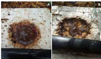
Figure 5: Some of the tested delivery devices had low permeability and resulted in water pooling on top of the substrate, causing Decoy to spill out.
