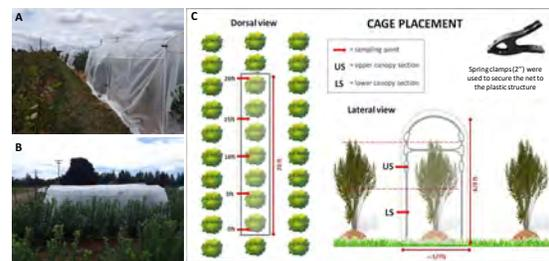
Figure 6: Cages used in the field trials. A, B) Each cage consisted of a PVC pipe structure enclosed by a fine mesh (0.8 mm). The piping was inserted over rebar hammered into the ground. Spring clamps secured the net on the structure (2"). C) Schematic drawings of the net cage show the size of the structures and the locations of the sampling points (red arrows).
