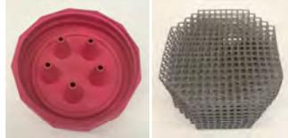
Figure 3: Examples of 3D-printed prototypic release devices developed to deploy Decoy in the field. Most of these devices did not prevent desiccation of Decoy and were abandoned.
