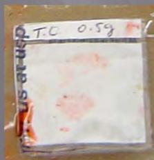
Fig. 1 Thyme oil is encapsulated by CD and placed in a Tyvek sachet allowing for CRP which is humidity dependent.
