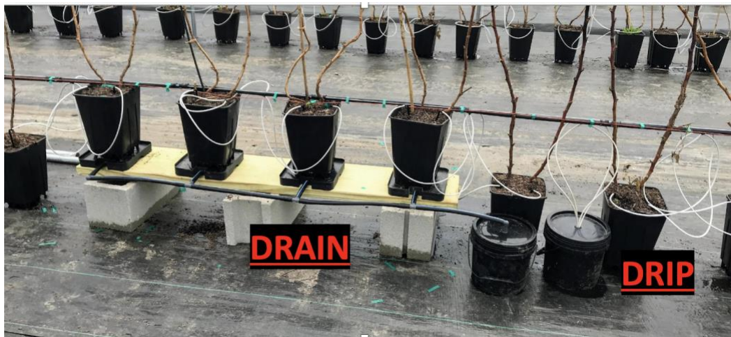
Figure 3 Monitoring station used to track fertigation input (drip) and pot leachate (drain) on a daily basis.
